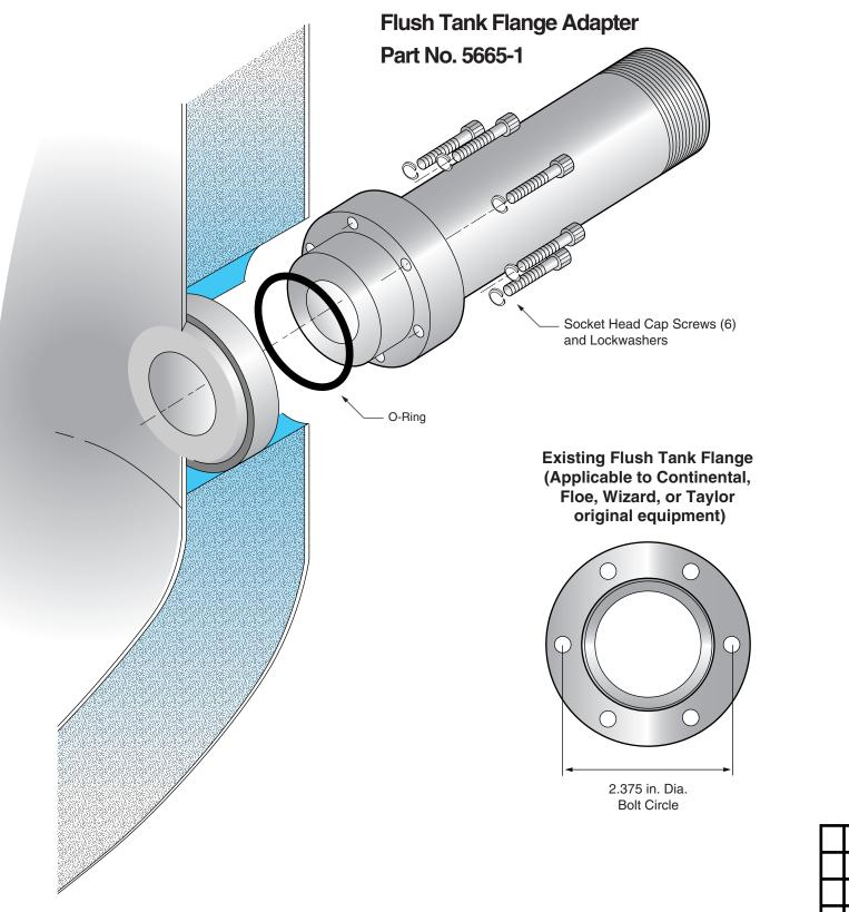
The complete adapter package supplied includes O-ring seal, socket head cap screws, lockwashers and 5/32 hex key wrench.
