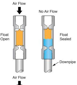
The Model 6563 Downpipe Check Valve is well suited for use on downpipe systems employing KING-GAGE Purge Control or LiquiSeal Purge Control liquid level transmitters. Hydrostatic pressure measurement using a downpipe (also known as a bubbler system) is a proven tank gauging technique that is both accurate and reliable.
