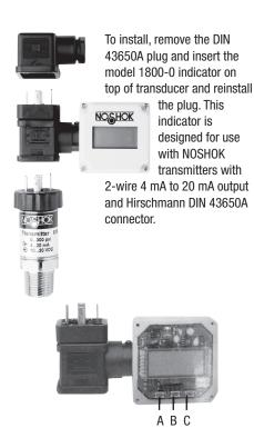
To program, first remove the cover from the indicator housing and identify the buttons A, B, and C. These buttons are used to program the indicator to match the pressure range of the transmitter.
